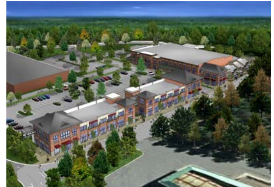
This picture illustrates how a large retail center can avoid being a “strip” center. Parking is behind the building, office uses are on the second floor, and windows make the building transparent.
